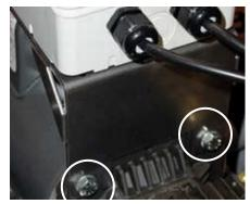
2. Mount bracket on motor using the two top pump bolts.
