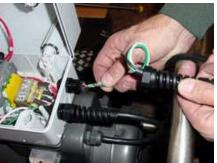
8. Insert the power cord into the box through the right side strain relief and hand tighten.
