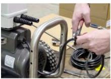
3. Cut the power cord at 21" from motor strain relief.
