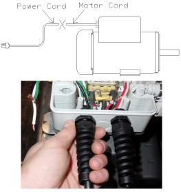
5. Insert the motor cord into the box through the left side strain relief and hand tighten.
