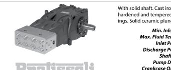
With solid shaft. Cast iron pump body with stainless steel manifold. Crankshaft is nitrided, hardened and tempered alloy steel. Forged steel connecting rods with anti-friction bearings. Solid ceramic plungers.
