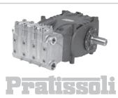
With solid shaft. Cast iron pump body with stainless steel manifold. Crankshaft is nitrided, hardened and tempered alloy steel. Forged steel connecting rods with anti-friction bearings. Solid ceramic plungers.
