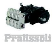
The MW Series Triplex Plunger Pump is available in 6 flows. The incorporated gearbox is available in 3 ratios, 1500, 1800 and 2200 rpm. It has double pressure packings, vertically fitted suction/delivery valves, splash lubrication and includes optimal drain/priming valve kit. Includes external gearbox posionable on left or right hand side of pump. Please specify RPM and gear box position when ordering.
