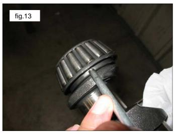
The new bearings can be mounted cold with a press or rocker, supporting it on the lateral surface of the ring nuts involved in press fitting with the rings. The press fitting operation can be facilitated by heating the involved parts to a temperature between  $120^{\circ}$  -  $50^{\circ}$  ( $250^{\circ}$  -  $300^{\circ}$ ), ensuring that the ring nuts go down to end stroke in their seats.
