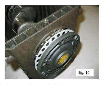
Once the type and number of shims have been determined using the table, check the following: assemble the shim pack on the indicator side cover centring (fig. 15), secure the cover to the casing, following the procedure in para. 2.1.2 and tighten the screws to their recommended torque.
