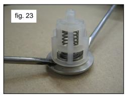
Disassemble the suction and outlet valve units, screwing a sufficiently long M8 screw in such a way as to be able to reach the valve plate and extract the valve guide from the seat, fig. 22, pos. 1. If the M8 threaded holes should not be present on the valve guide, dismantling can be easily carried out by leveraging with simple tools fig. 23.
