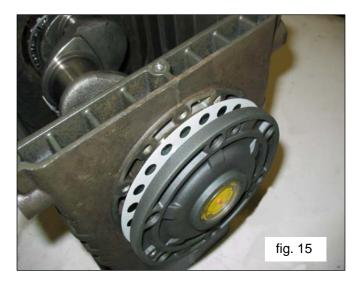
Once the type and number of shims have been determined using the table, check the following: assemble the shim pack on the indicator side cover centring (fig. 15), secure the cover to the casing, following the procedure in para. 2.1.2 and tighten the screws to their recommended torque. Check that the shaft rotation stall torque is between 4 Nm and 6 Nm.
