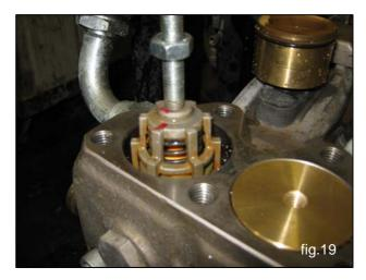
Dismantling of the suction and outlet valve units can be carried out screwing in a sufficiently long M10 screw which can move the valve plate and remove the valve guide from the seat (fig. 20); pos.1. If the threaded holes should not be present on the valve guides, dismantling can be easily carried out by leveraging with simple tools fig. 21.
