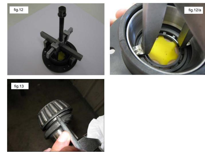
The new bearings can be mounted cold with a press or rocker, supporting it on the lateral surface of the ring nuts involved in press fitting with the rings. The press fitting operation can be facilitated by heating the involved parts to a temperature between  $120^{\circ} - 50^{\circ}$  ( $250^{\circ} - 300^{\circ}$ ), ensuring that the ring nuts go down to end stroke in their seats.
