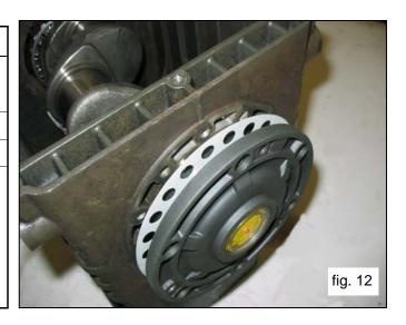
Insert the shims under the cover on the sight glass side (see fig. 12), fixing it to the crankcase using the appropriate screws, and verifying that the stall torque is between 4 Nm and 7 Nm.
