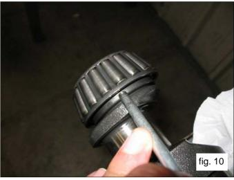
The new roller bearing can be mounted at room temperature with a press or fly press; it is necessary to lay them on the lateral side of the relevant ring nuts with apposite rings. The driving operation can be facilitated by heating the relevant parts at a temperature ranging between 120° - 150° C (250° - 300° F), making sure that the ring nuts are correctly fitted into their seats.
