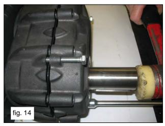
Remove the reducer case cover and extract the bearing from the pinion using standard tools (fig.15) Remove the ring gear fastening screws with the related washer, and extract the ring gear. If necessary, use a slide hammer applying it to two M8 holes (pos.①, fig.16), or a standard extraction tool (fig.16).
