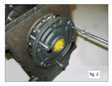
Push the piston guides and connecting rods forward in order to facilitate the lateral extraction of the pump shaft. Two marks are visible on the crank shaft ①, as shown in fig. 3 and in fig. 3/a; they must be turned towards the operator in order to facilitate extraction.
