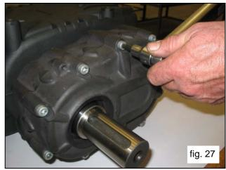
Verify the conditions of the sealing lip of the pinion oil wiper; replace if necessary using the tool cod. 27904800.
