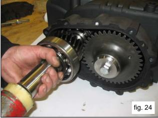
The bearings and the ring gear may be mounted at room temperature. The driving operation could be facilitated by heating the interested parts to a temperature ranging between 120° - 150°C (250° - 300° F), being sure that the ring nuts fit thoroughly into their seats.
