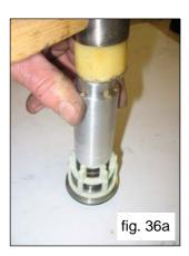
Insert the suction and delivery valve units checking that are thoroughly inserted in the head seat. Therefore apply the valve covers and proceed with calibrating the related M12x35 screws with a torque wrench as indicated in Chapter 3.
