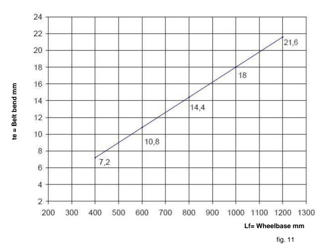
Conclusion: with a wheelbase of 600 mm and with a dynamometer, loading the belt branch with 75 N as indicated in fig 12, a "te" bend of approximately 10.8 mm is obtained.
