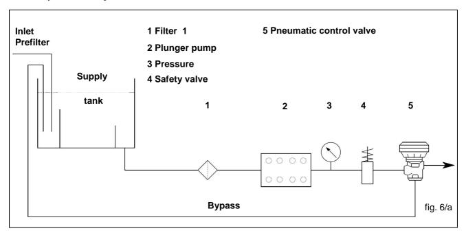
The filter must be installed as close as possible to the pump, it must be easily inspected and must have the following characteristics:
