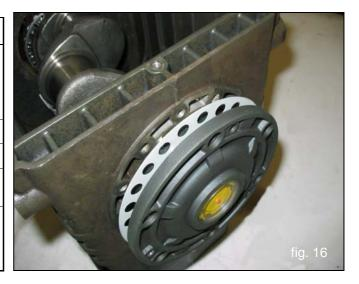
Insert the shims under the cover on the sight glass side (see fig. 16), fixing it to the crankcase using the appropriate screws, and verifying that the stall torque is between 4 Nm and 7 Nm. If the torque value is correct, connect the rods to the crankshaft; otherwise, redefine the shims again repeating the operations.
