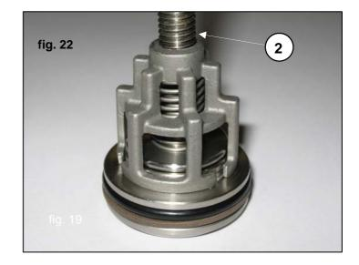
Disassemble the suction and delivery valve units by screwing on an M8 screw long enough to act on the valve and extract the valve guide from the valve seat, pos. 2 (fig. 22).
