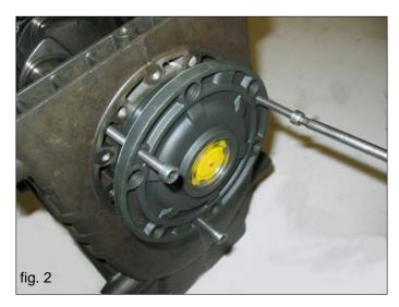
Push the piston guides and connecting rods forward in order to facilitate the lateral extraction of the pump shaft.
