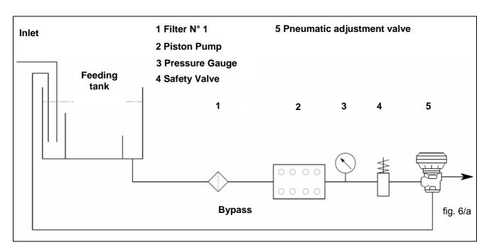
The filter must be installed as close as possible to the pump, should allow easy inspection and have the following characteristics:
