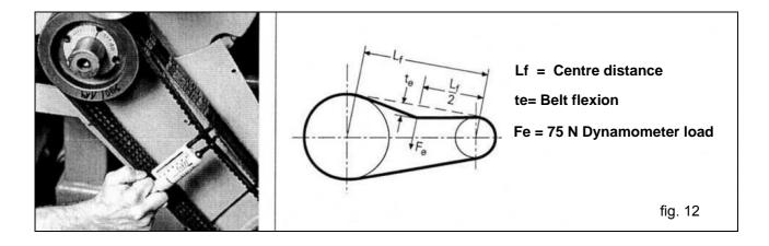
$N.W_1$ . If not differently indicated by the belt Manufacturer, the inspection of the correct tension value, and the related tension adjustment if needed, is to be carried out after at least 30 minutes of operation in order to obtain belt settling. The best efficiency and maximum duration is obtained with the correct tension value.
