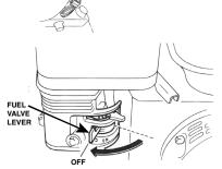
3.3 Turn the fuel valve to the OFF position.
