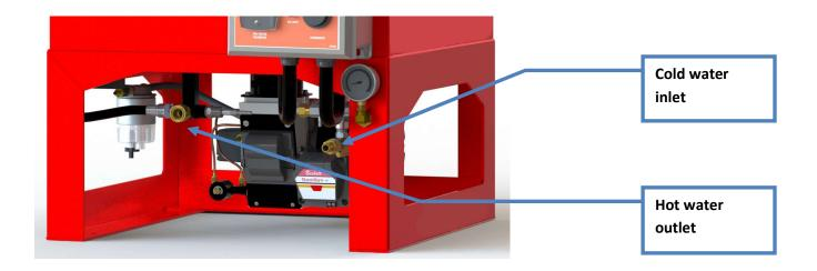
Connect the outlet of the high pressure pumping unit to the cold water inlet of the heater module
