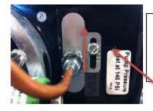
MOVE ELECTRODE ASSEMBLY DOWN BY PULLING GENTLY ON COPPER TUBE NUT. THIS MOVEMENT WILL REPOSITION THE INDICATING LINE UP ONE NOTCH ON THE ADJUSTER PLATE. TIGHTEN NUTS.
