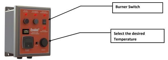
b) Be sure water can flow to the heater coil before turning on burner switch. Start the pumping unit involved until a steady stream of water is flowing from the spray gun (holding the spray gun open. Turn burner switch to "ON" position. Burner will ignite and remain in operation as long as there is sufficient water flow to satisfy the flow switch and temperature limit control. To shut off main burner, turn burner switch to "OFF".
