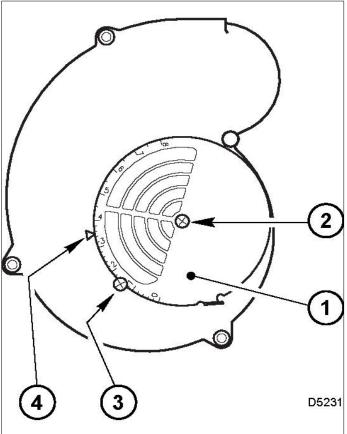
**C)** The final position of the air adjustment plate will vary on each installation. Use instruments to establish the proper settings for maximum  $CO_2$  and a smoke reading of zero.
