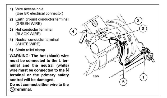
The burner may be controlled using either a DIRECT LINE VOLTAGE control circuit (120V AC 60 cycle) **OR** a LOW VOLTAGE control (24V AC 60 cycle) using a R8038A Honeywell switching relay or equivalent.
