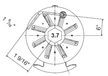
**IMPORTANT:** Do not turn the ignition electrode. Leave it as shown in the drawing. If the ignition electrode is put near the ionization probe, the amplifier of the control box may be damaged.
